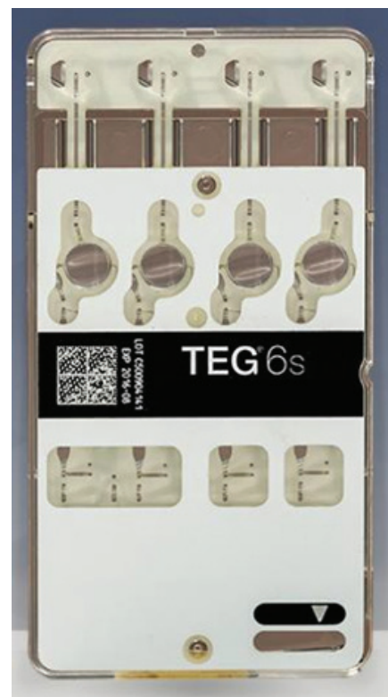
Figure 2. TEG® 6s cartridge - There are four channels in the TEG® 6s cartridges – CK, CKH, CRT and CFF.
